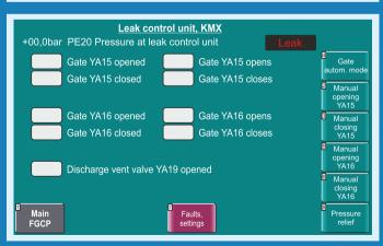
The automation system performs monitoring of gas parameters and control of shutoff valves' electric drives and solenoid valves
